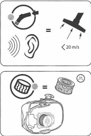
Detail 4: LED indicator: flow rate & filter warning
