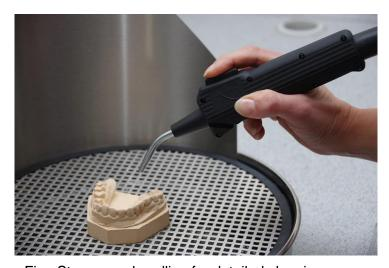
Fig.: Steam gun handling for detailed cleaning
