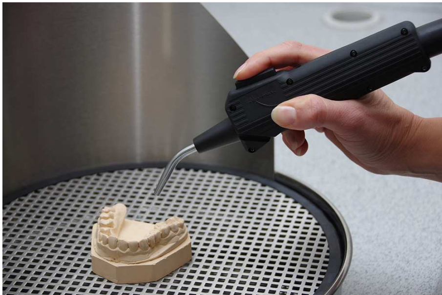
Steam gun position for detailed use on objects and holding position downwards
